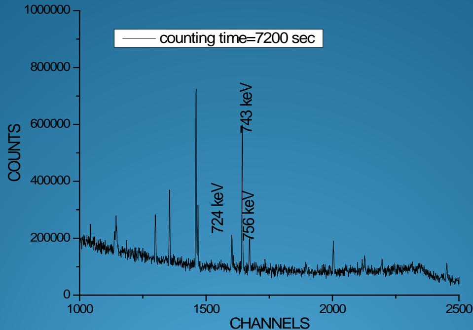
The gamma-ray spectra, as shown in Fig. 1, were analyzed with peak fitting program PHAST which can search for up to 500 peaks and fit model peak shape.
